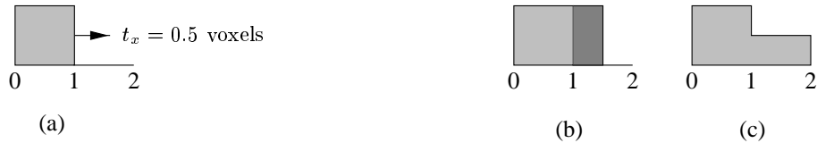
Fig. 4. Schematic 1D diagram illustrating volume estimation by linear interpolation of a binary image. Shown in (a) is a voxel of unit intensity with neighbours of zero intensity. Translating one edge by 0.5 voxels increases the volume by 50%, shown as a dark grey region in (b). The neighbouring voxel is interpolated with an intensity of half a unit (c). Hence the measured volume will be 1 voxel in (a) and 1.5 voxels in (c).
